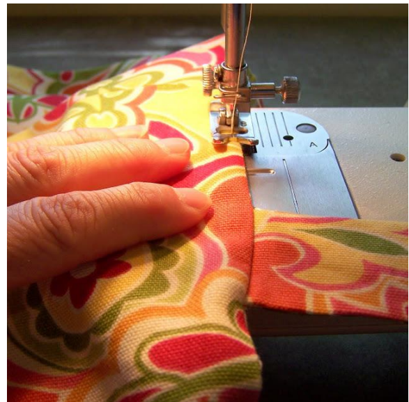
21. Top-stitch around the top edge. First stitch 1/8" from the edge and then repeat at 1/2" from the edge.
